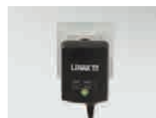
Electronic switch mode power supply unit integrated immediately after the mains plug
